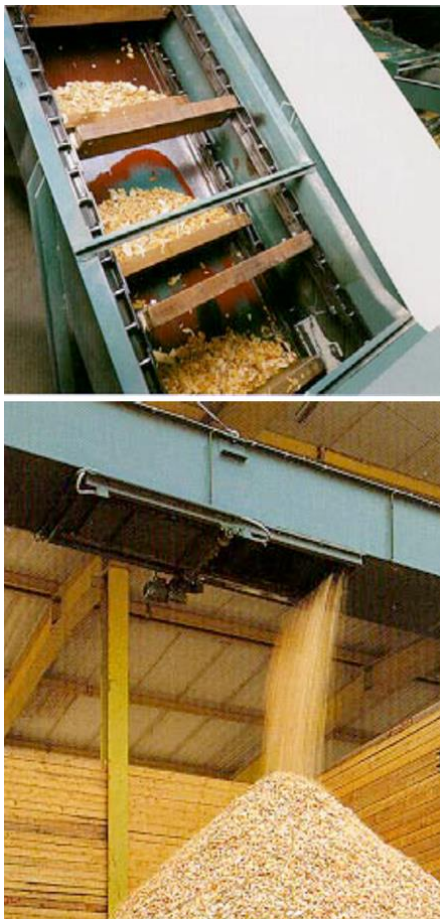
Figure 6.33 Scraper chain conveyor [69].
