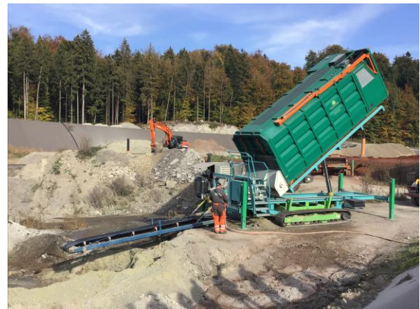
Figure 9.2 Dust-free depositing of wood ash into a landfill (source: Amstutz Holzenergie AG/Holzenergie Schweiz).
