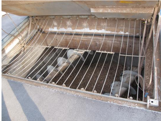
Figure 6.11 Filling screws (source: Holzenergie Schweiz).
