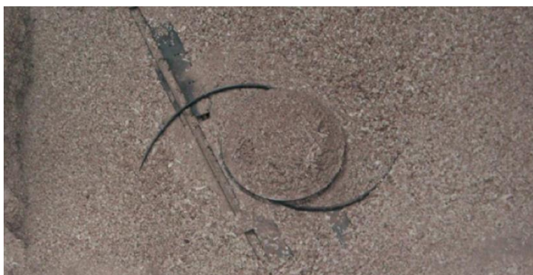
Figure 6.28 Spring core discharge (source: Herz).
